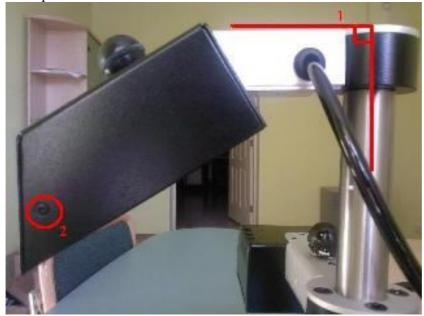
3) Adjust the laser to be as near as possible to the center. Tight the laser fixing screws back.
